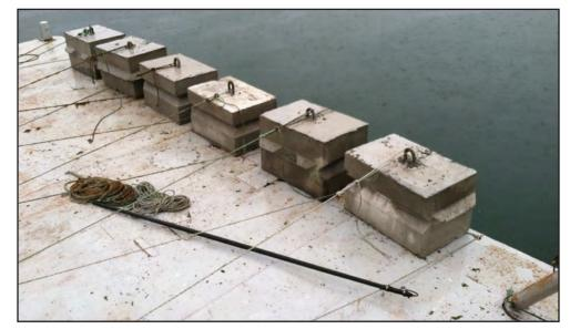
Figure 1.5 Concrete block moorings
