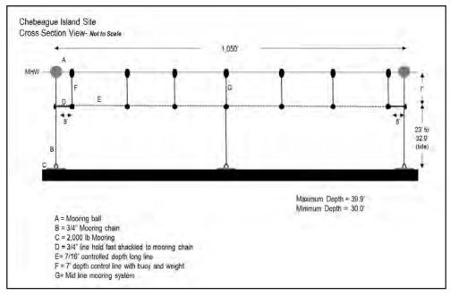
Figure 1.3 Farm design cross section view
