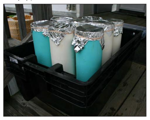
Figure 5.3 Settling tubes and spools packed for transport before ice is added around tubes
