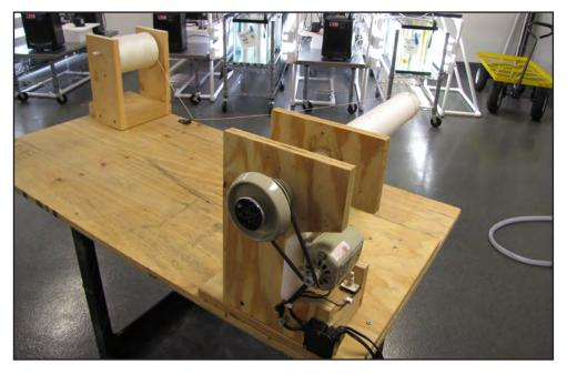
Figure 2.11 A handmade spool winder, using a sewing machine motor as the power source
