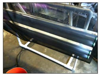
Figure 2.4 Fine mesh screen used to create light levels of 20 µmol m <sup>-2</sup> s <sup>-1</sup>
